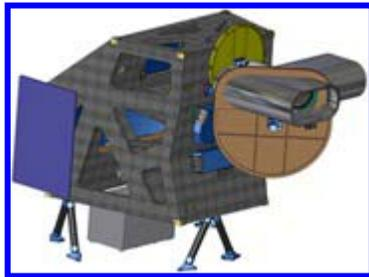
past Landsat sensors using a technical approach demonstrated by a sensor flown on NASA's experimental EO-1 satellite. OLI is a push-broom sensor with a four-mirror telescope and 12-bit quantization. OLI will collect data for visible, near infrared, and mid infrared spectral bands as well as a panchromatic band. It has a five-year design life. Figure 12 compares the OLI spectral bands to Landsat 7's ETM+ bands.
