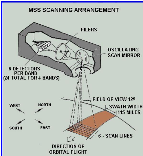
**FIGURE 7: Multispectral Scanner System**
