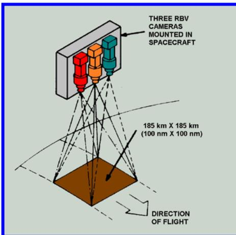
The RBV camera system was designed to obtain high resolution television pictures of the Earth. Three cameras were used to take pictures simultaneously in three different spectral bands. The cameras were similar except for the spectral filters contained in the lens assemblies to provide separate spectral regions. Camera 1 covered the visible blue-green portion of the spectrum, Camera 2 the visible orange-red portion, and Camera 3 the red-near-infrared portion. They were designated Bands 1-3.
