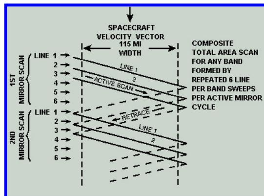
**FIGURE 8: Scan Track Direction**
