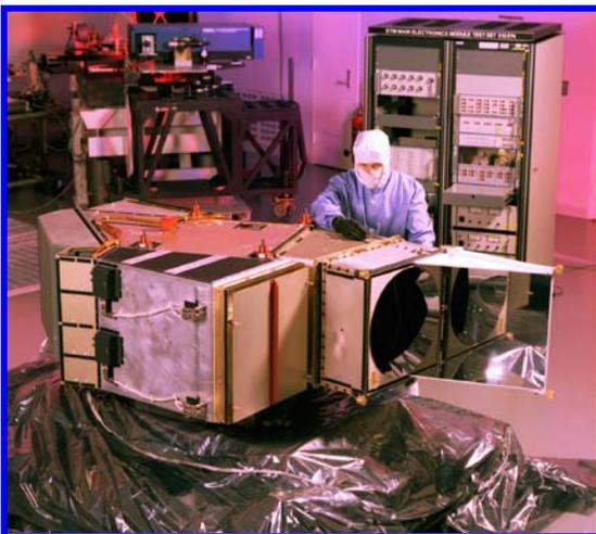
**FIGURE 11: Engineer with the Landsat 7 ETM+ instrument.**
